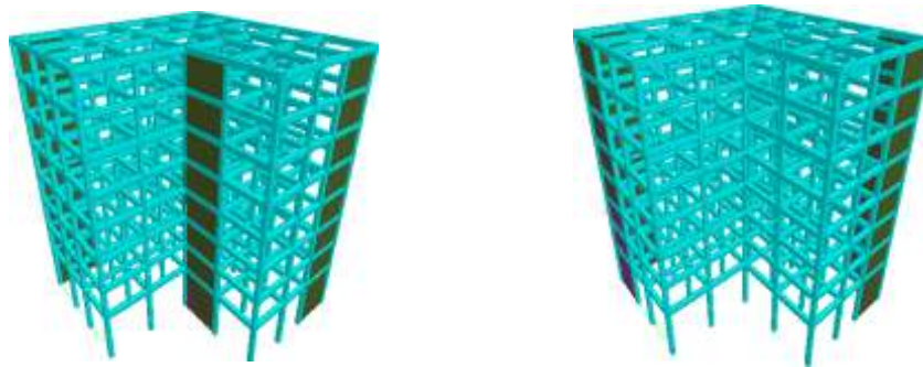
(a) Model-1 (b) Model-2 Fig. 4:- 3D of Models with Shear Walls.
