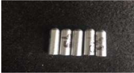
Fig.9. Specimens for wear testing
