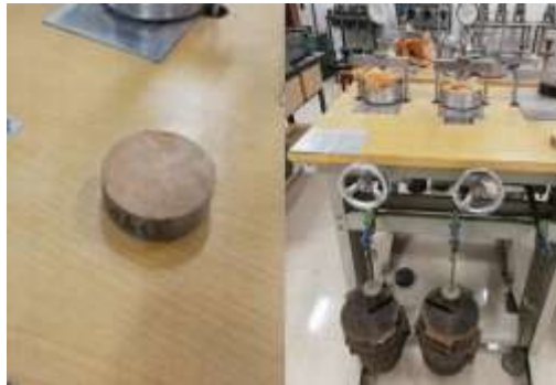
7Fig.7 Samples and test process diagram of confined compression test
