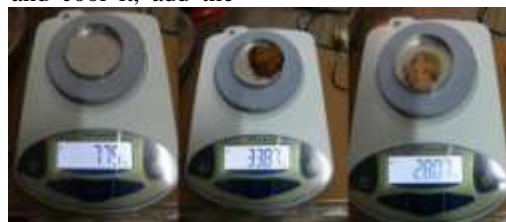
Fig .5 Water content test process
