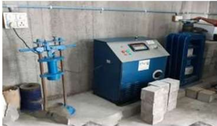
Fig- 3.14 Testing of cube CTM
