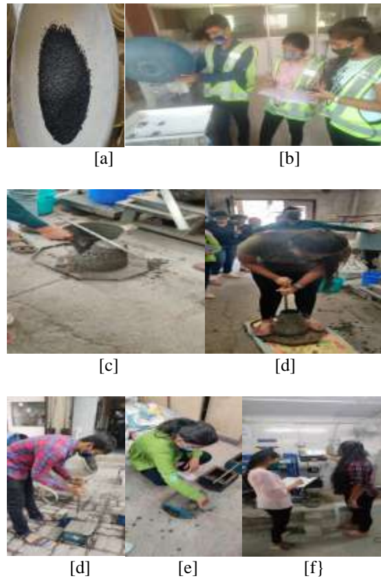
(Fig1) [a] Preparation of crumb rubber [b] Weighing of crumb [c] Slump cone test [d] Tamping [e] Casting of cube [f] Testing of cube.
