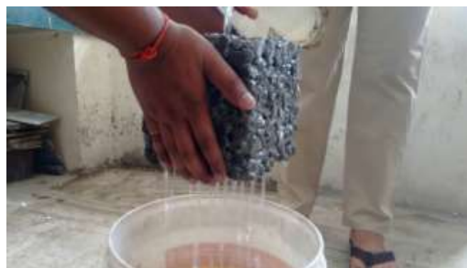
Figure 1.1: Water Draining Through Pervious Concrete
