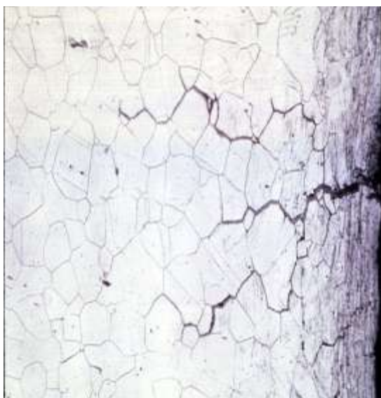
Figure 1.7: Intergranular corrosion of stainless steel
