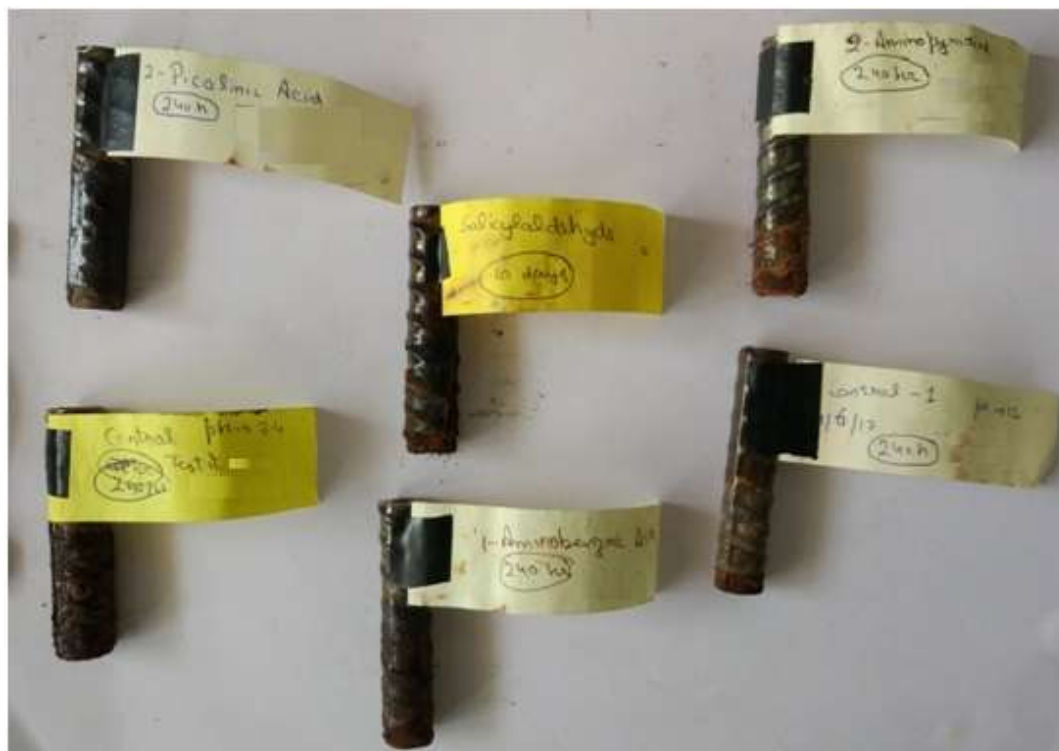
Figure 5.8: After 240 hours of immersion in various solutions, steel samples were tested for half-cell potential and linear polarisation resistance.
