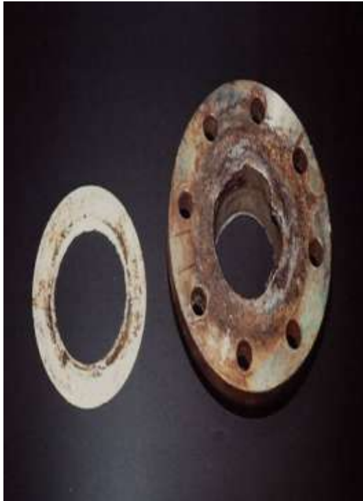
Figure 1.4: Crevice corrosion on a stainless steel flange
