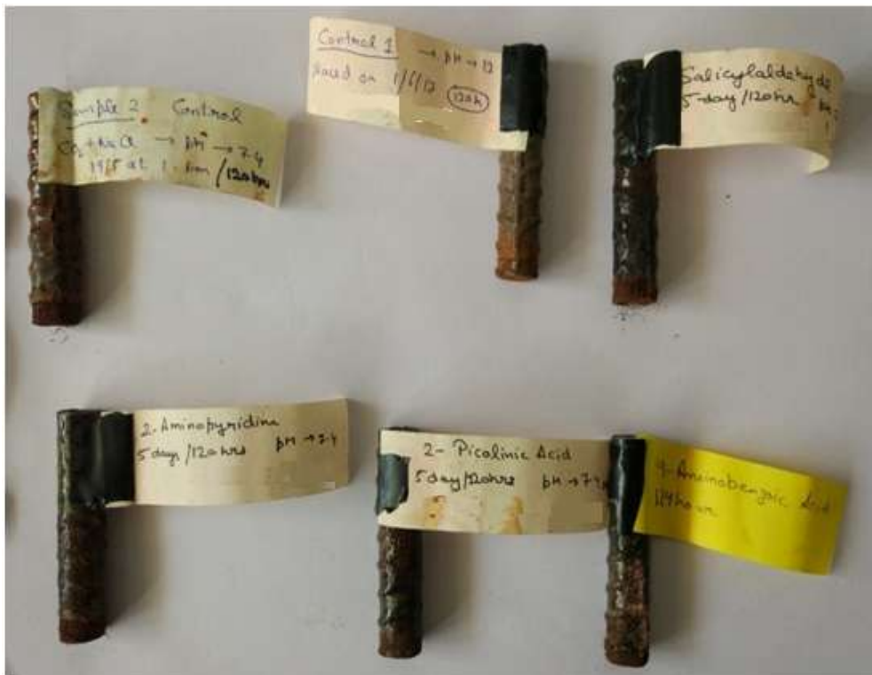
Figure 5.6: Steel specimens after measuring Half-cell Potential and Linear Polarization Resistance, immersed in different solutions after 120 hours
