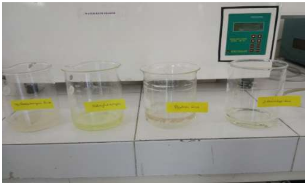
Figure 4.4: Solutions of Chemical Inhibitors in Carbonated Saturated NaCl
