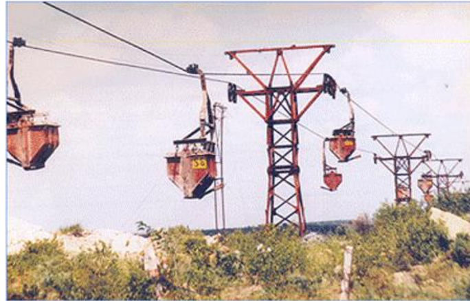
Figure: Ropeway carrying Bauxite to Lohardaga Station.
