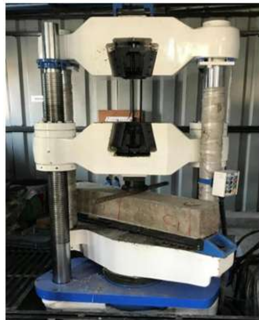
(Fig No. 4 Experimental setup of concrete beam)
