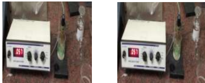
Fig Electrical Conductivity Apparatus
