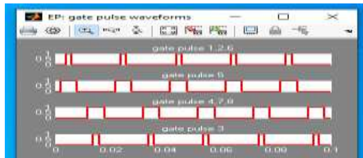
Fig 11(a1): Gate pulse for five level inverter: EPPWM
