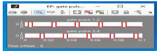
Fig 10(a2): Gate pulse for three level inverter: PDPWM
