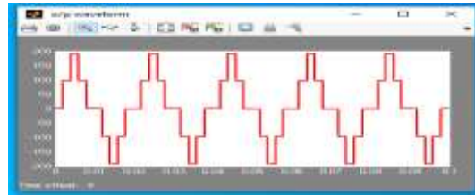
Fig 11(c): Five level Output waveform
