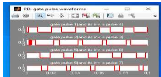
Fig 11(a2): Gate pulse for five level inverter: PDPWM
