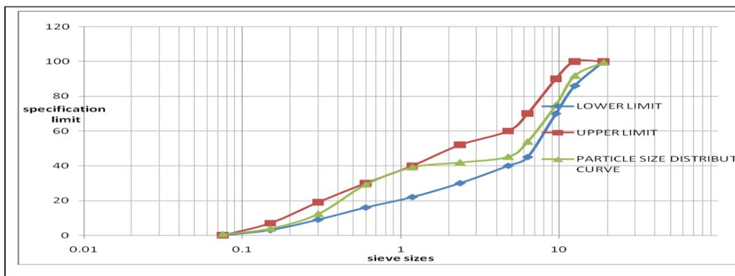
Figure 1: Aggregate Gradation Curve
