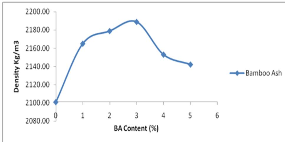
Figure 4: Variation of Density (Kg/m<sup>3</sup>) with Modifier Content
