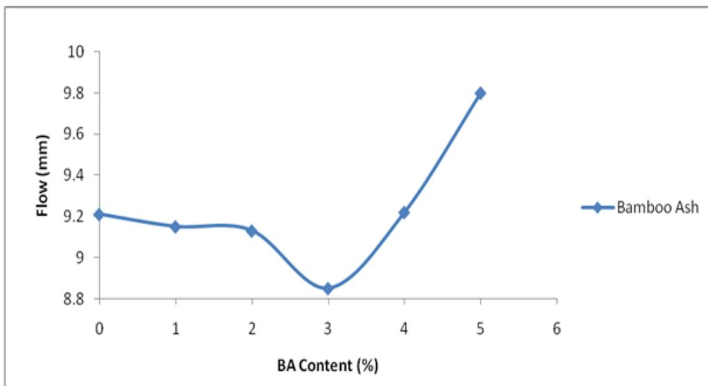
**Figure 3:** Variation of Flow (mm) with Modifier Content
