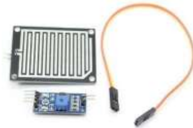
Fig6: RAIN WATER SENSOR HUMIDITY SENSOR
