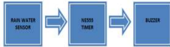
Figure 1: Block Diagram of a Simple Rain Detector which Uses IC 555 Timer
