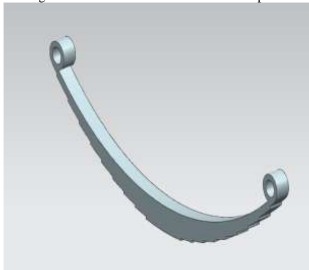
Figure:3.4 CAD model of coconut fibre and S Glass fibre composite leaf springs
