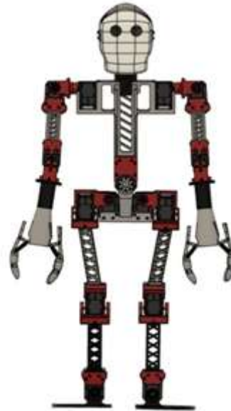
Fig 18: 3D CAD of Full Skeleton structure of Humanoid Robot
