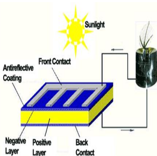
Figure (3) Typical solar cell structure.
