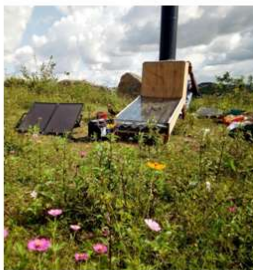
Figure 1 (b): Pictorial view of the constructed dryer under test condition.
