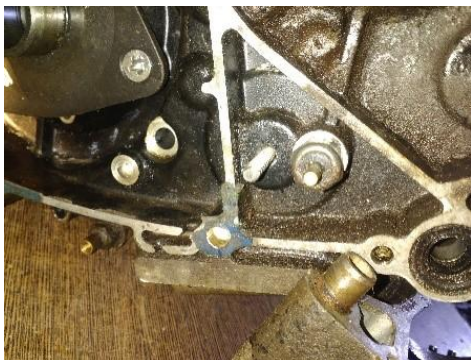
(A) External view of gearbox after installing modified gear shift drum.
