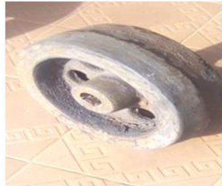
plate ii: casting after fettling
