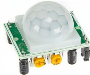
Plate 4. PIR motion sensor [9]
