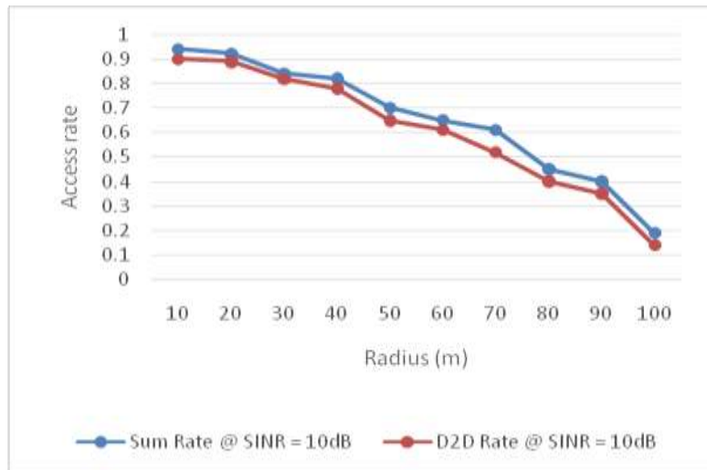
Figure 4.0: Access rate of system when the minimum SINR was 10dB with CUEs = 25 and DUEs = 15 for uplink scenario.
