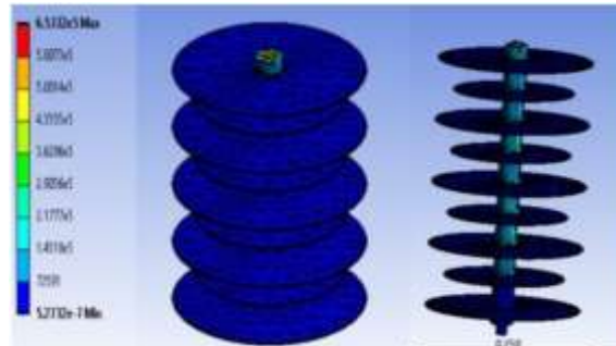
THE ELECTRICAL FIELD DISTRIBUTION OF ALTERNATE SHED
