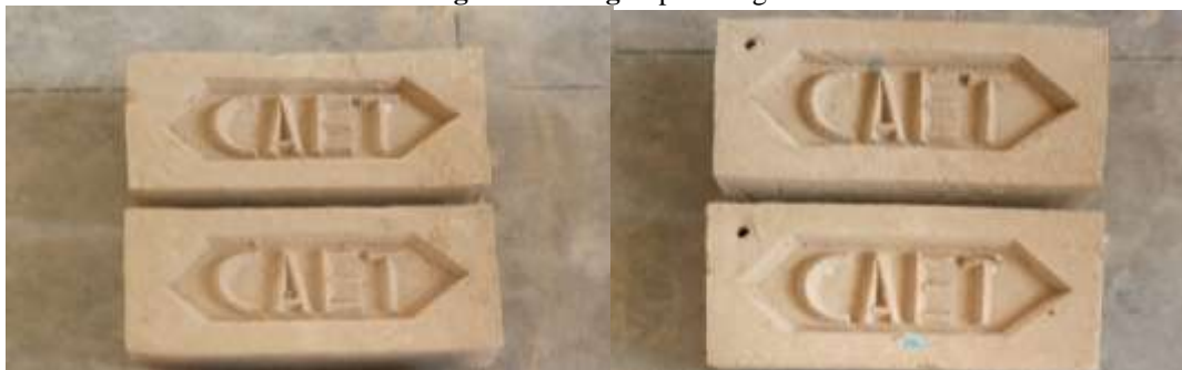
Ratio 100:0 brick, 100% clay Ratio 95:5 brick, (95% clay & 5% plastic)
