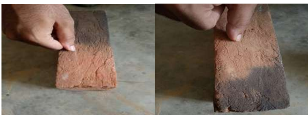
(c) 90 % clay 10 % plastic brick (90:10)(d) 85 % clay 15 % plastic brick (85:15)
