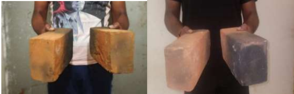
(a) 100 % clay brick (100:0) (c)90 % clay 10 % plastic brick (90:10)
