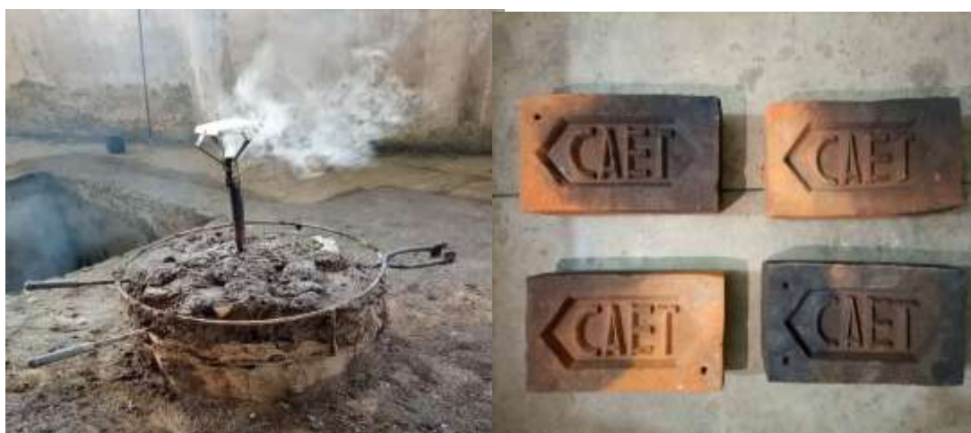
Fig.5 Laboratory-Furnace Fig. 6 Laboratory-furnace burnt brick
