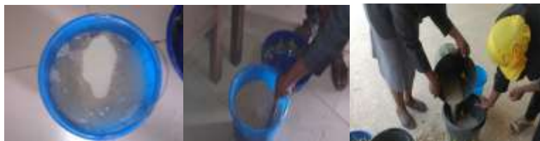
Fig. 9: Sedimentation and decantation process
