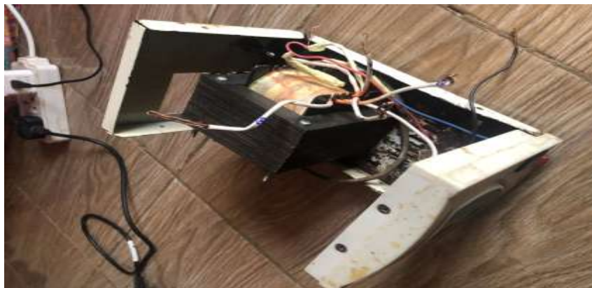
Plate 2.1: Assembling of Constructed Step-up Transformer.
