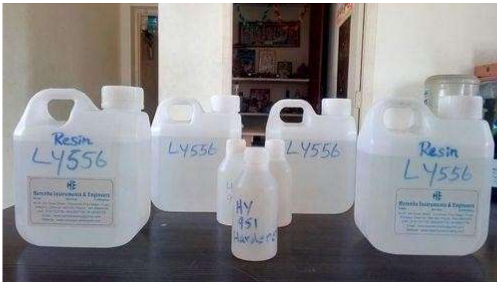
Fig 3.3 Epoxy Resin (LY556) and Hardner (HY951)
