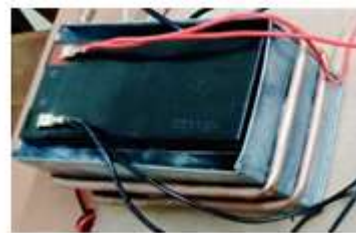
Fig. 3 Liquid Cooling by using copper tube
