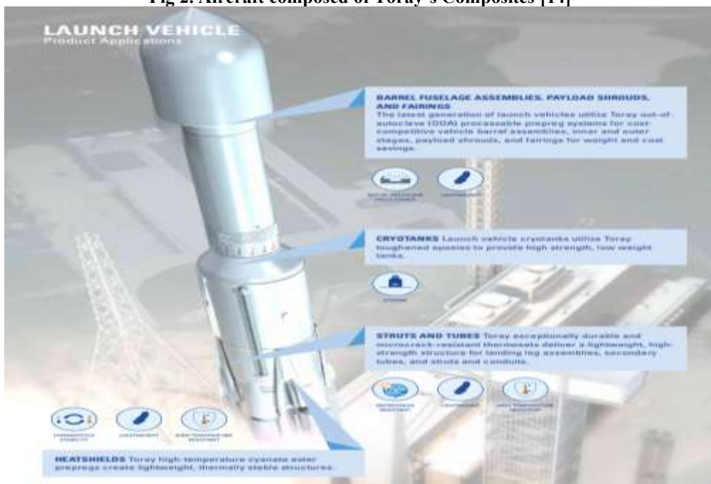
Fig 3. Launch Vehicle Composed of Toray's Composites [14]
