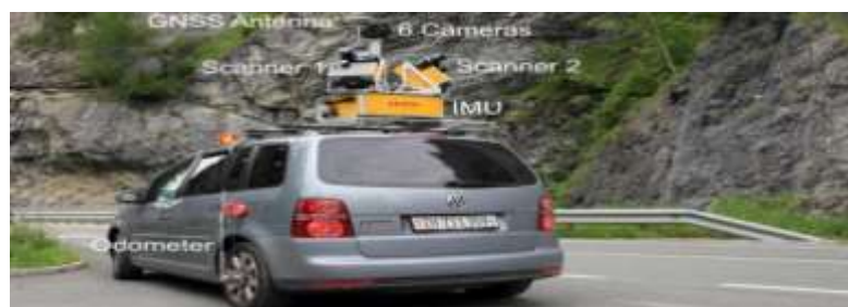
Figure 3. Mobile mapping system mounted on a car
