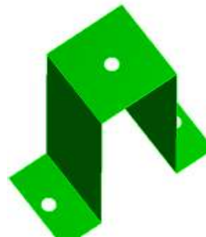
Fig.15: GFRP bracket mass: 235gram
