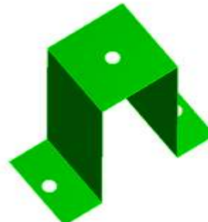
Fig.14: Steel bracket mass: 923gram
