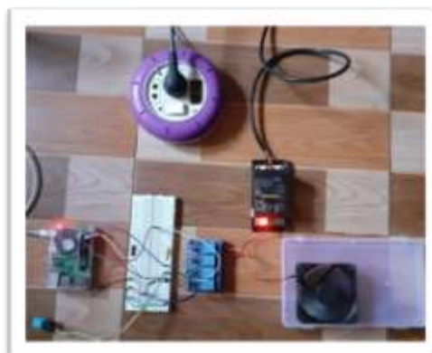
Fig .3 DHT11 sensor interfacing with raspberry pi.
