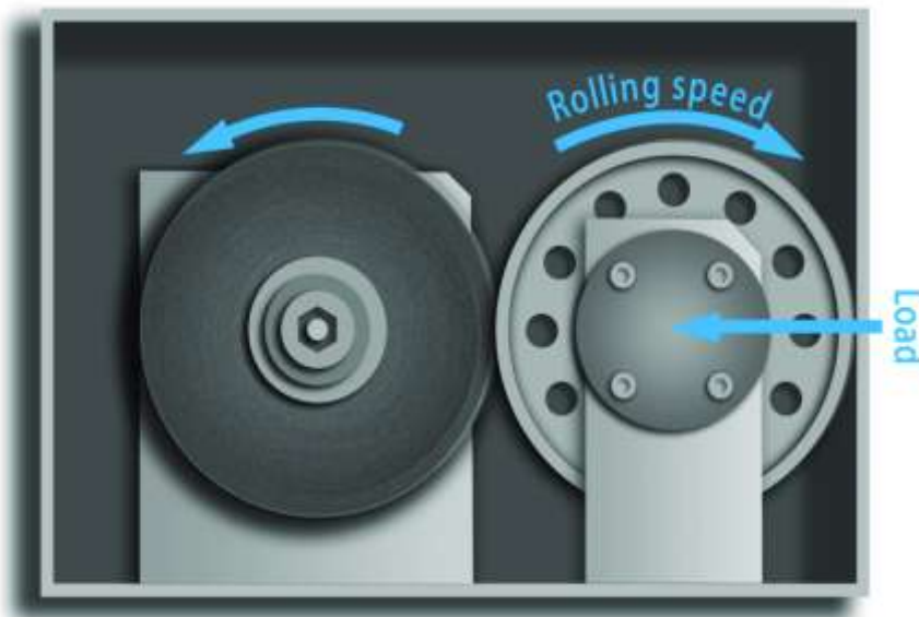
Fig.6 –Tire LSP test machine schematic diagram
