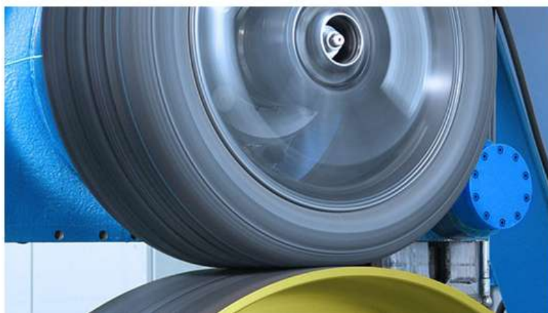
Fig.5 –Tire endurance testing setup
