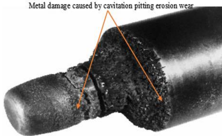
Figure 3.11: Cavitation erosion wear damage of a globe valve trim (Sotoodeh, 2015).
