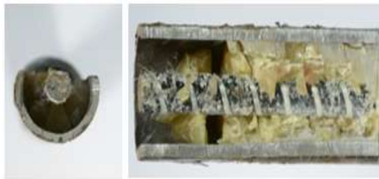
Fig.9 BFRP bar ends in the steel tube anchors after tensile test
