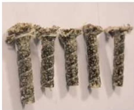
Fig.11. Typical failure mode
