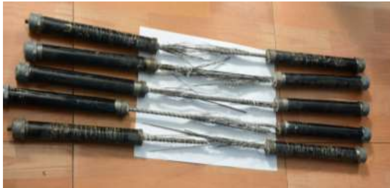
Fig. 8BFRP Rupture Failure of tensile specimens
