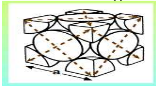
Plate II: FCC Crystal Structure
