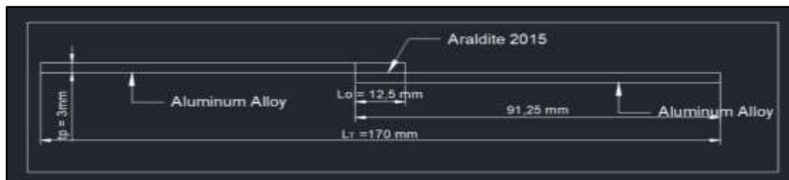
Figure 5.1: Shape and characteristic dimensions of single-layer connection model
