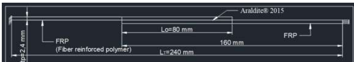
Figure 5.2: Dimensions and specific geometry of the single-lap joint model
