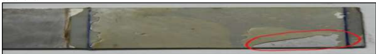
Figure 6.5.1: The specimen shown above failed due to cohesion failure
