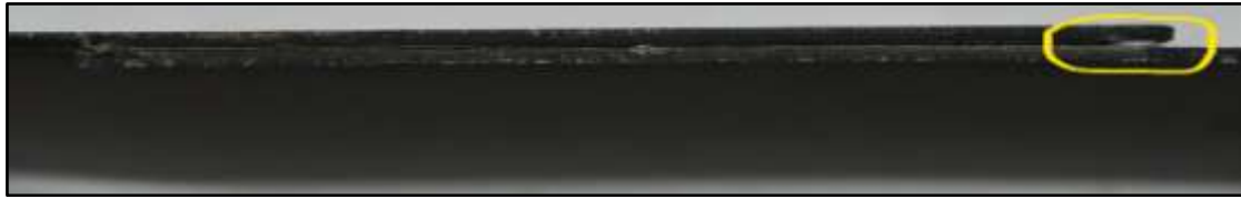
Figure 6.5.4: The specimen shown in the figure above failed in Mode 1, also known as the Opening mode, in which the fracture starts perpendicular to the crack plane. A bend or pressure application may be the cause of this.
