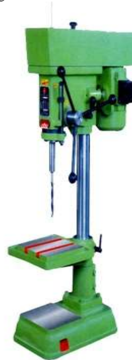
Figure 1. Conventional Pillar type drilling machine
