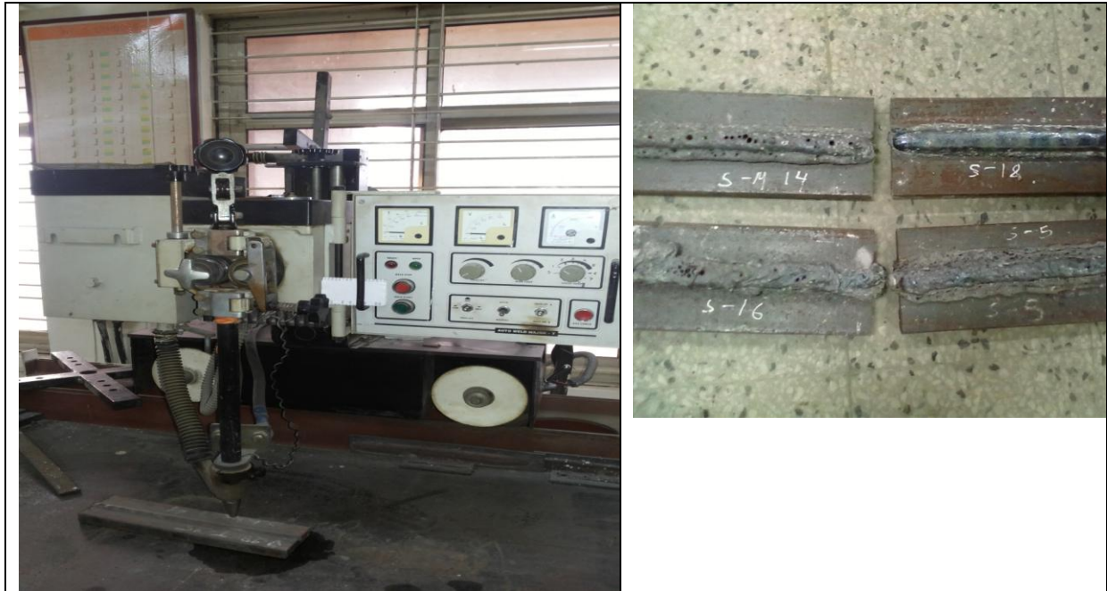
Figure 1. The SAW Machine used for welding
