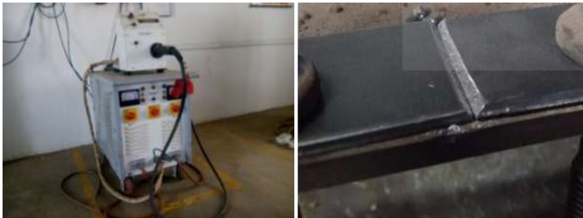
Figure 1 Front View of MIG welding Setup and Sample Preparation for Butt Welding Joint
