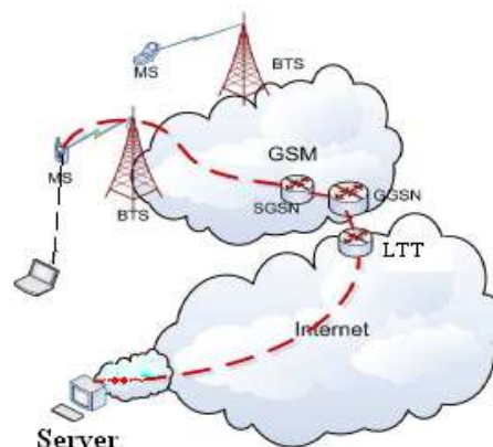
Fig.1: Network measurement System
