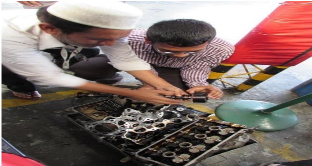
Figure 10: Engine Overhauling (Navana Toyota 3S Center).
