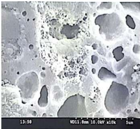
Fig 3. SEM analysis of QBSCC of w/b ratio 0.4
