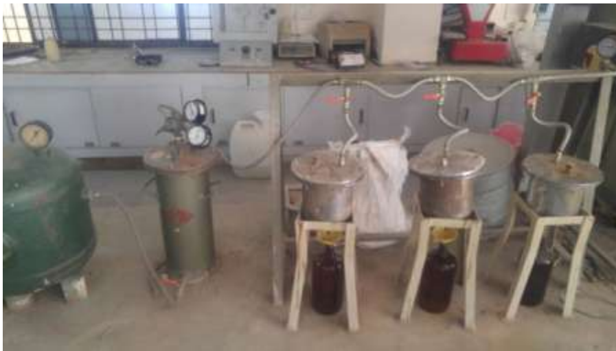
Fig 5. Water Permeability test set-up
