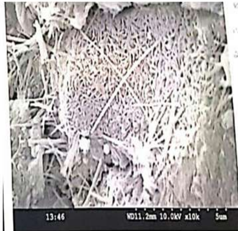
Fig 2. SEM analysis of QBBSCC of w/b ratio 0.3
