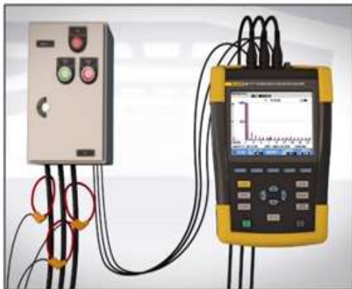
Figure 7: Power and motor analyzer connecting to a motor feeder circuit.
