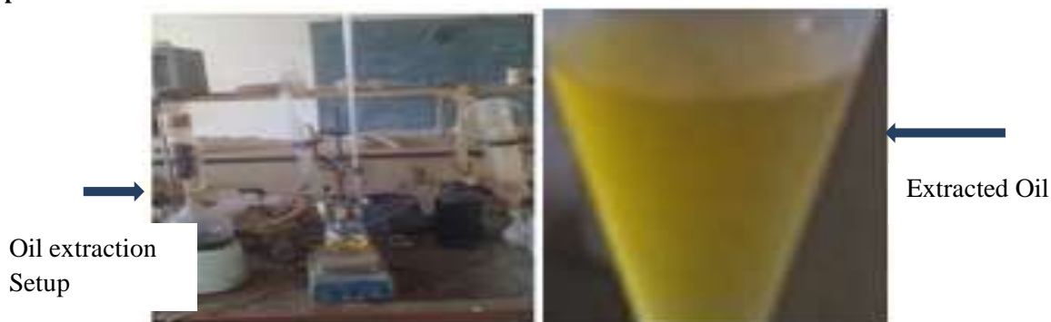
Plate II: Setup for oil extraction and sample of oil extracted from sweet orange seeds
