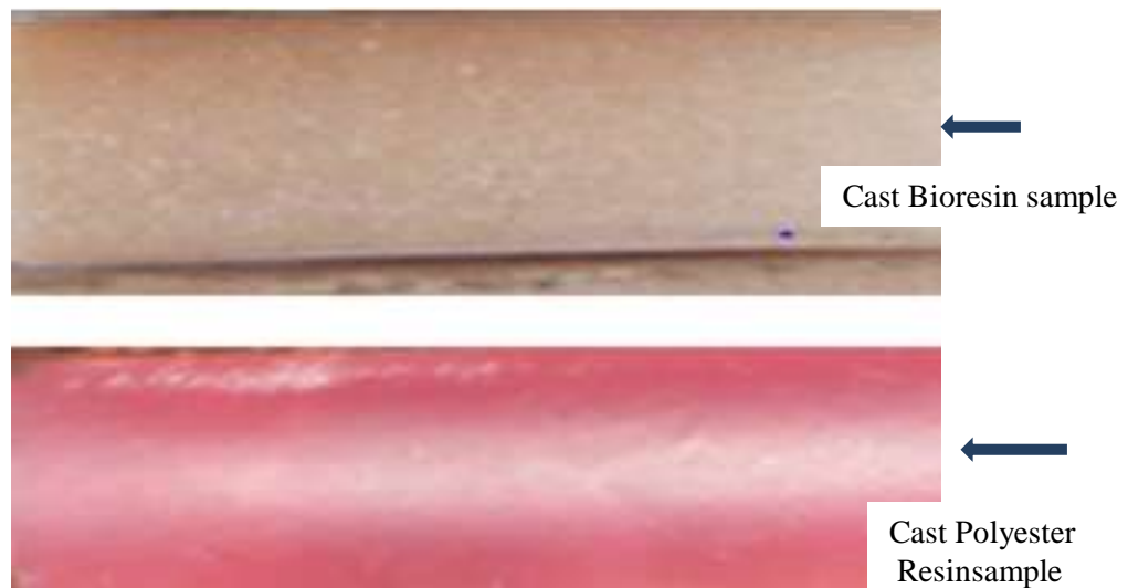
Plate V: Sample of cast bioresin from sweet orange seeds and cast polyester
