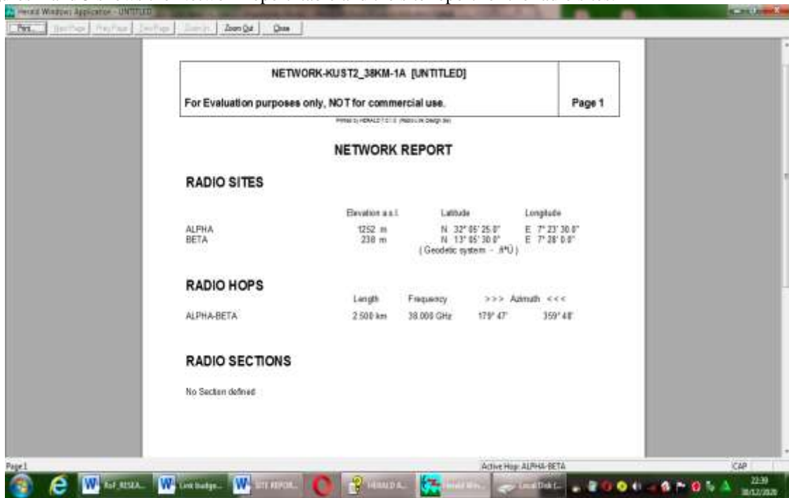
Figure 4: Network report for radio sites ALPHA (32°05'',7°23''); BETA (13° 05''N, 7° 28''E at 38GHz,2.5Km range.
