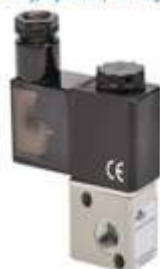
3-way, 2-position, normally closed direct-acting solenoid valve, spring return
