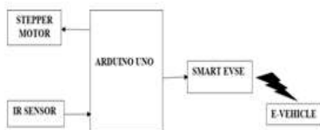
Fig. 1, Smart parking part WIRELESS CHARGING PART:
