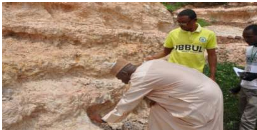
Fig. 5. Conducting textural examination on the clay deposit at Kutigi. Geochemical results show that this clay deposit (top-most layer 3) has the best quality (highest alumina and least silica content) amongst the clay deposits studied
