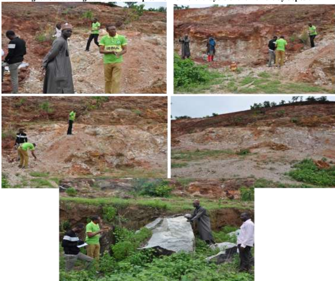
Fig. 7. Mapping, logging and sampling of the Kwakuti alumina-rich clay (top 4 pictures) and marble deposits (the boulder) (bottom picture)
