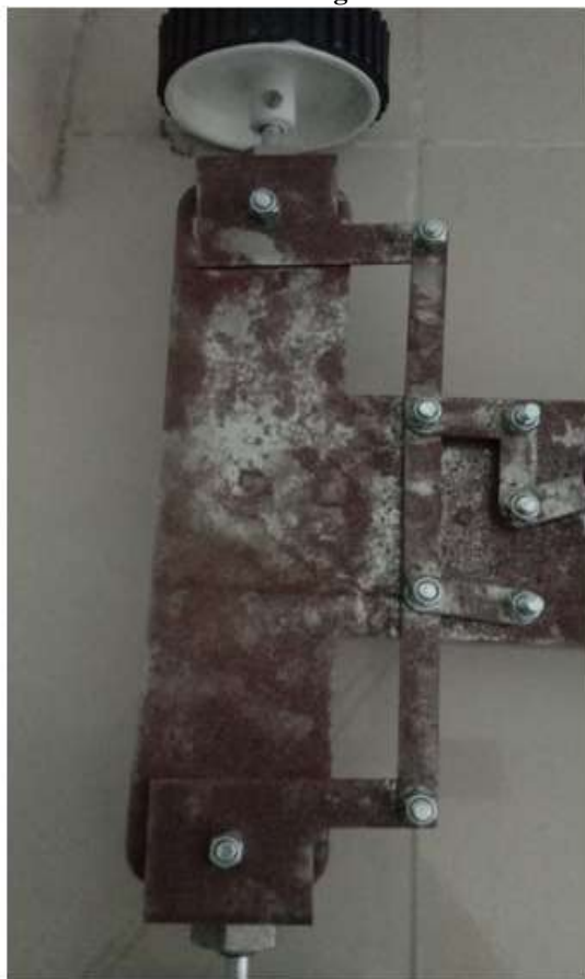
Fig.c Ackerman Steering Linkage System
