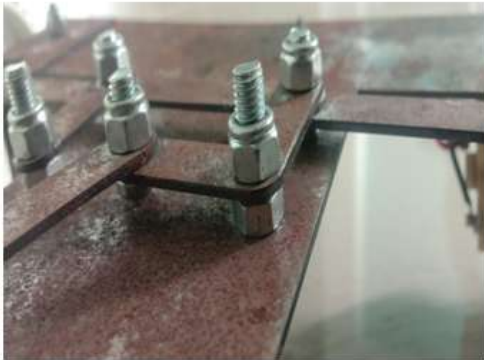
Fig.b L type Link that moves Ackerman Steering
